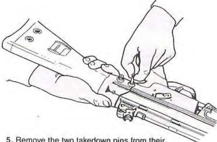
Remove the two takedown pins from their storage holes in the buttstock and insert them in their proper holes from left to right at the rear of the receiver. The SAR-3 is now fully assembled.
